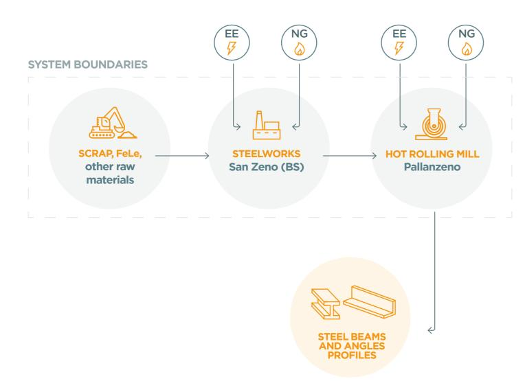
The process begins in **San Zeno** with the **pre-processing of the external scrap**, which is purified from impurities and loaded into the melting furnace; ferroalloys give the metal bath the desired characteristics, after which the liquid metal is cooled in the form of a steel billet.
